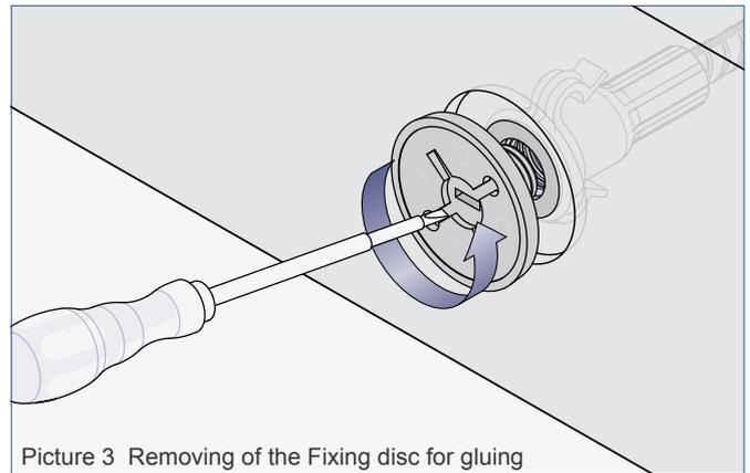
Picture 3 Removing of the Fixing disc for gluing
