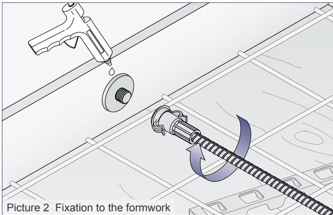
Picture 2 Fixation to the formwork
